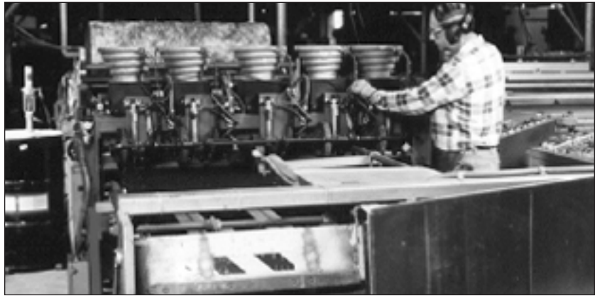
Shop fabricating fibrous glass duct liner
