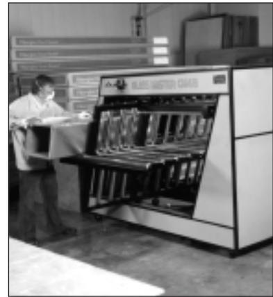
Completing duct section using closure machine.
