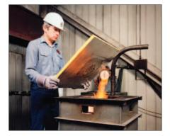
Test Procedure: The exterior surface of the fibrous glass duct material is subjected to a gas flame from a furnace. It must resist penetration of the test flame for 30 minutes while supporting a concentrated load of 2 pounds per square inch.
