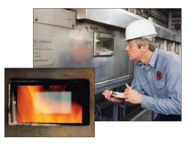
Test Procedure: The UL Surface Burning Characteristics test, recognized as a standard test for evaluating all types of building materials as to their performance when exposed to heat and flame, is conducted in a 25-foot tunnel, with fiber glass duct — including closure system forming the ceiling. When a gas flame impinges on the duct material, it must not exceed a flame spread rating of 25. Smoke developed must not exceed a rating of 50.
