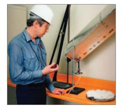
Air ducts should not continue to burn progressively, and exterior surfaces of the material should not drop particles that are capable of igniting combustible materials such as cotton.
