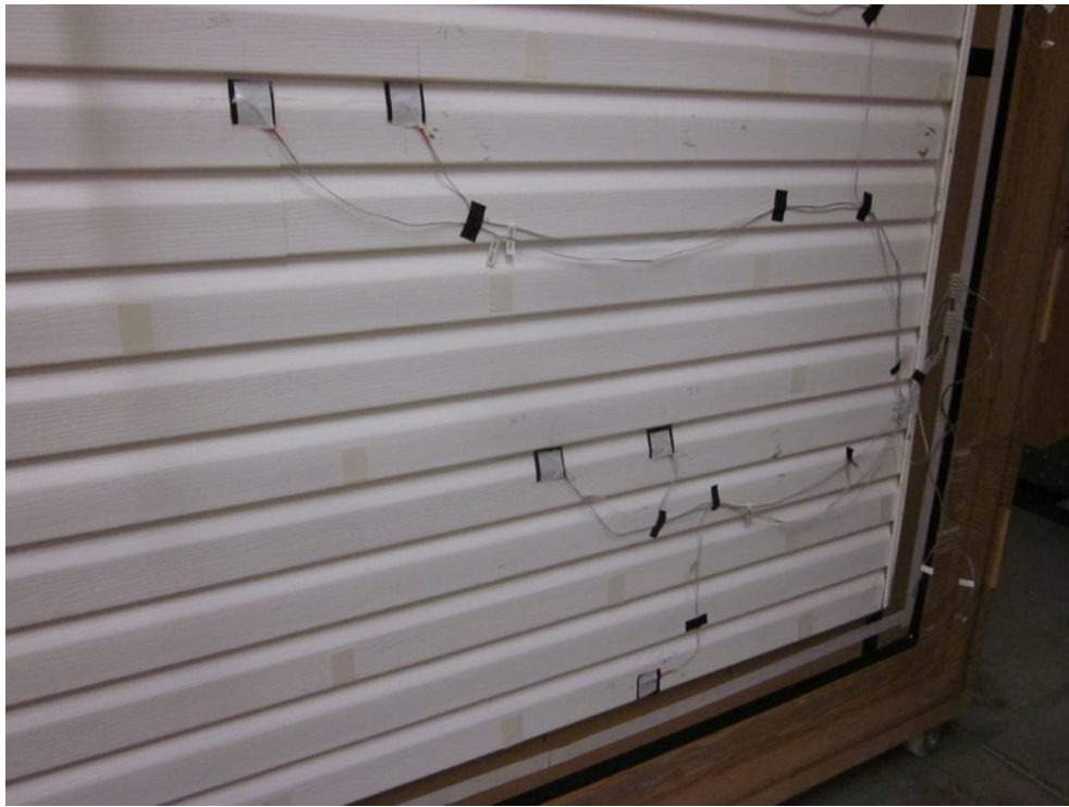
Figure 26 – Climate Box Side, Tape Grid
