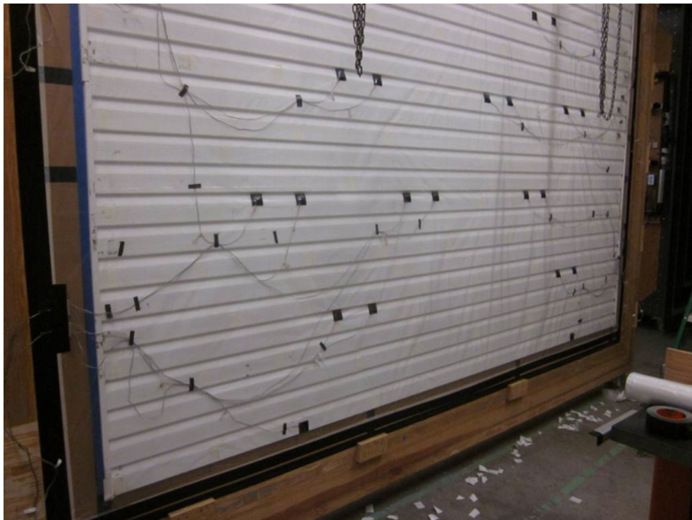
Figure 27 – Climate Box, Polyethylene Installed
