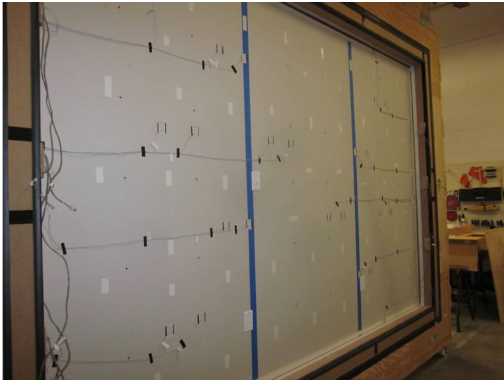
Figure 24 – Meter Box Side, Grid of Double-Sided Tape
