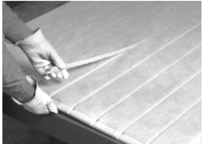
Fig. 3-34A. Removing scrap from grooved duct board.
