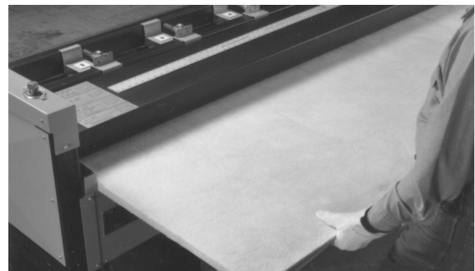
Fig. 2-9. Feed duct board into machine, female shi lap edge first, left hand edge firmly against guide, parallel to rollers. Turn on machine and guide board as friction rollers pick it up and pull it through the cutting tools.
