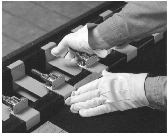
Fig. 3-31A. Duct board grooving machine set up for cutting ten-sided fibrous glass duct.
