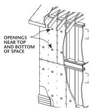
Exterior application of sidewall insulation is accomplished by removing sections of the exterior siding, making holes in the sheathing and blowing insulation in to fill the stud spaces. In both cases, it is recommended that a professional insulation contractor with knowledge of general framing principles should be hired to do the job.
