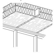
As mentioned earlier, loose-fill can be installed to any R-value. Because R-values per inch vary by product, always check the manufacturer's recommended installation instructions and install the proper amount. Inches alone may not determine R-value.
