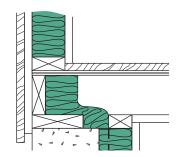
For unfinished basements that contain furnaces, water heaters, ducts, etc., manufacturers offer special basement wall insulation which is available in 4 ft. or 6 ft. widths in 50 ft. rolls. It comes with a white flame-resistant, polypropylene facing and is intended for use in applications where the insulation will be left exposed. It can be applied either full or half wall height.
