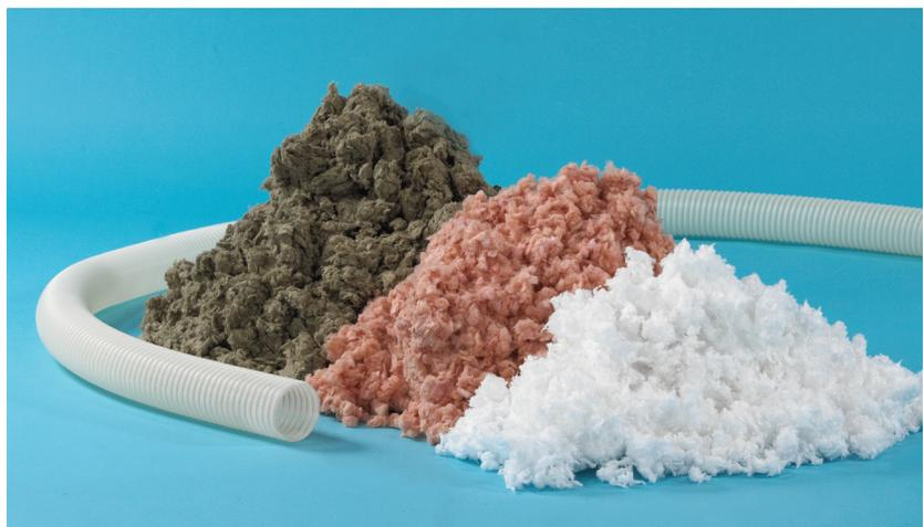
Loose-fill fiber glass, rock wool and slag wool insulation can be blown with most types of pneumatic machines and provide the R-value needed to meet the building codes. Once installed they work for the life of the building with negligible settling and no maintenance.
