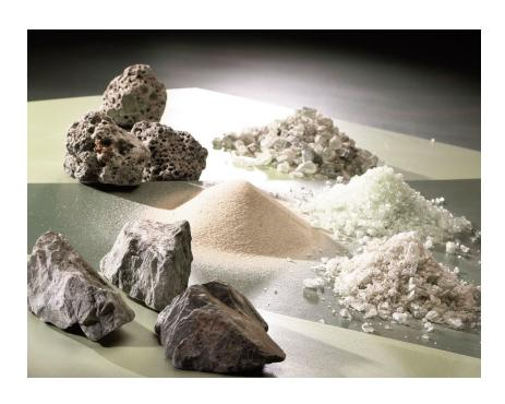
Fiber glass, rock wool and slag wool are made from a combination of natural and recycled ingredients such as basaltic rock, blast furnace slag, recycled glass cullet and sand. The natural ingredients, sand and rock, are readily available. The use of blast furnace slag and glass cullet are recycled materials that are transformed into a product that saves energy and reduces pollution.
