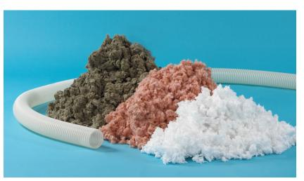
Loose-fill fiber glass, rock wool and slag wool insulation can be blown with most types of pneumatic machines and provide the R-value needed to meet the building codes. Once installed they work for the life of the building with negligible settling and no maintenance.
