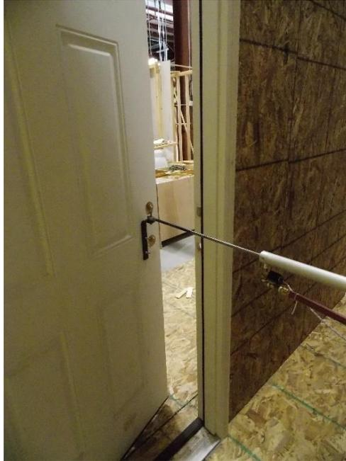
**Figure 6. Cylinder of Vibration Mechanism**
