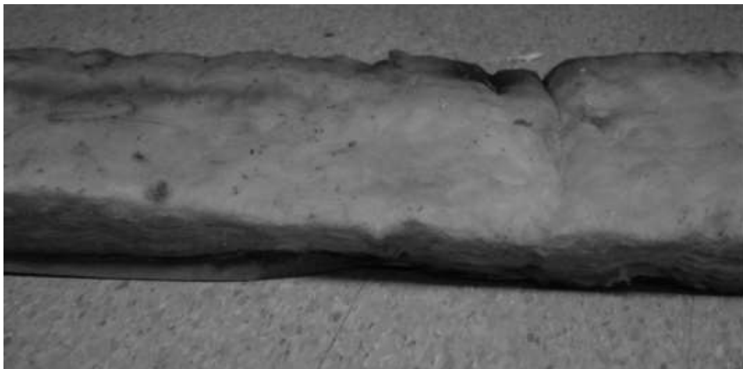
Figure 3 Sample No. 1 – R11 Faced Fiberglass Insulation
