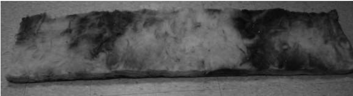
Figure 5 Sample No. 3 – R7 Faced Fiberglass Insulation
