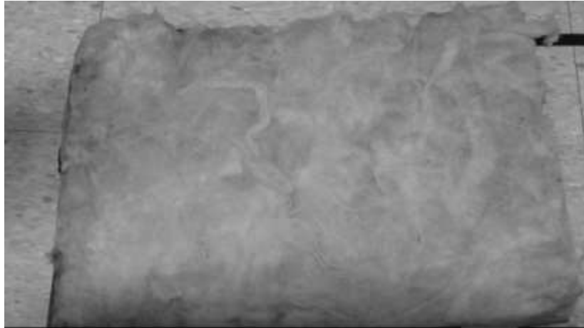
Figure 7 Sample No. 5 – R9.6 Faced Fiberglass Insulation
