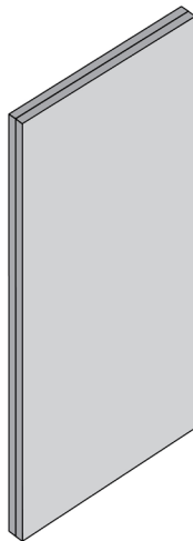
Two layers of drywall as a single panel
