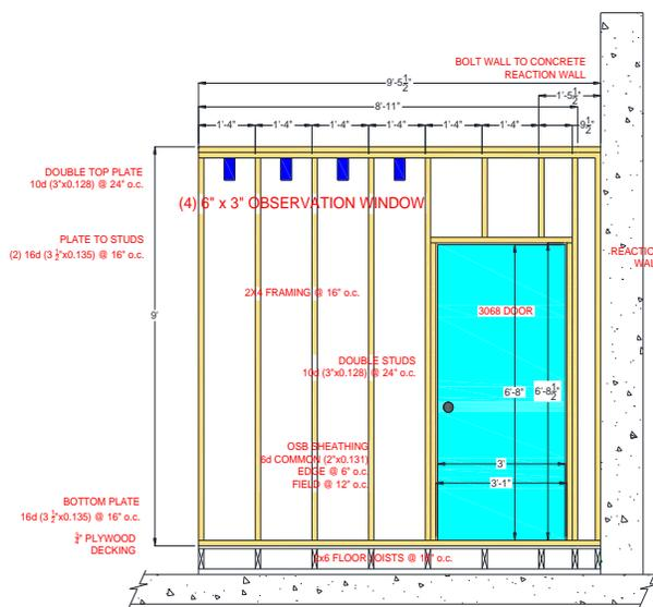
Figure 1. Wall Interior/Gypsum Side
