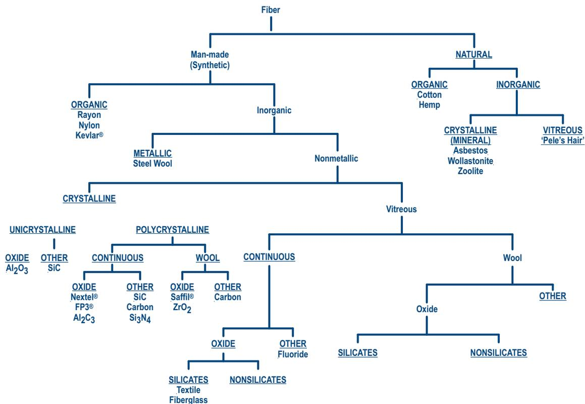
This classification scheme shows the very broad nature of synthetic fibers in contrast to natural fibers. This figure is valuable because it shows how SVFs are but a small part of the “family tree” of all synthetic fibers. But this
