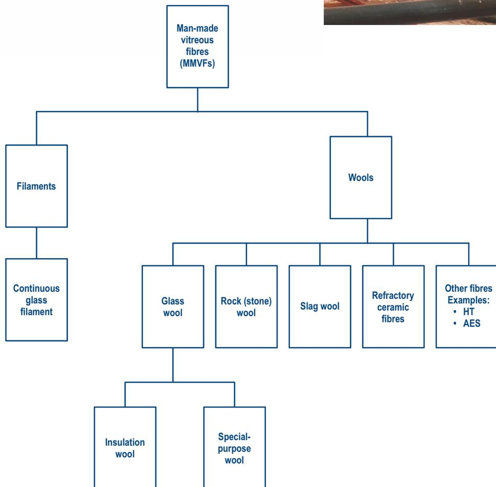
Within each of these categories, there are commercial products representing a range of compositions and durabilities. AES, alkaline earth silicate wools; HT, high-alumina, low-silica wools
