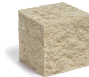
Spray foam insulation (Open or Closed Cell)
